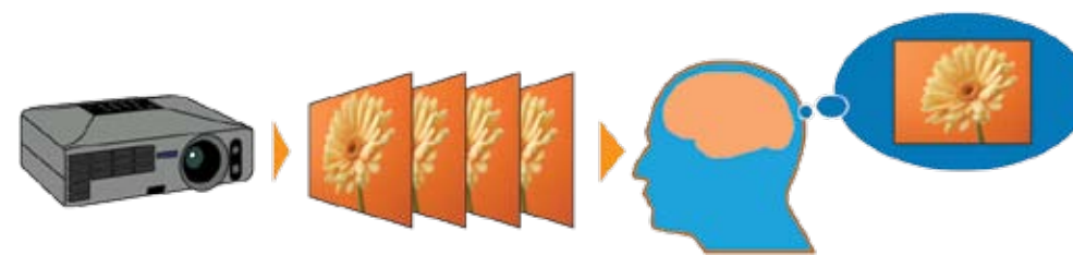
3LCD projector : RGB are projected at the same time, which makes the single composite image easy on the eyes.
